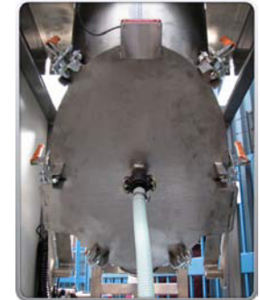
Quick release toggle clamps to access product chamber for cleaning and maintenance.
