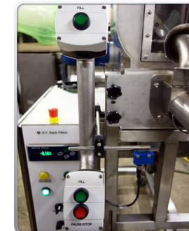
Hand start fill facility and no bag/no fill sensor for maximum safety.
