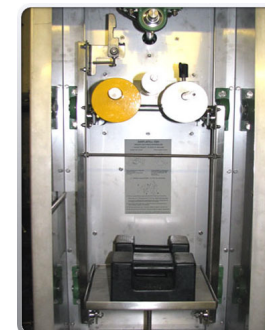
Internal mechanical weighing mechanism of the S1000GR.
