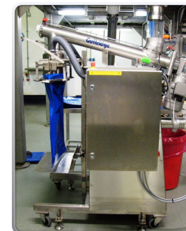
All screw feeders have a maximum 15 degree incline to reduce after flow and improve accuracy.
