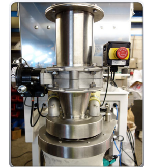
Integral butterfly valve to eliminate product after flow for a cleaner work place..
