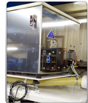
Flexible wall feeder mounted on optional load cells for a loss in weight system.
