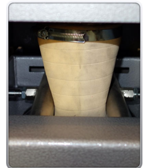
Pneumatic pinch valve assembly to control product feed flow rate.
