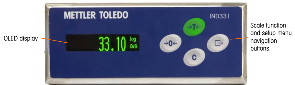
Figure 1-8: IND331 Front Panel Layout
