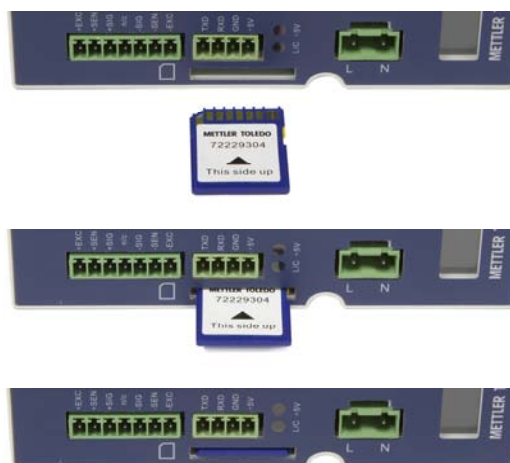
Figure 4-7: SD Memory Card Insertion, DIN Terminal
