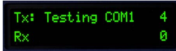
Figure 4-3: Serial Test Display
