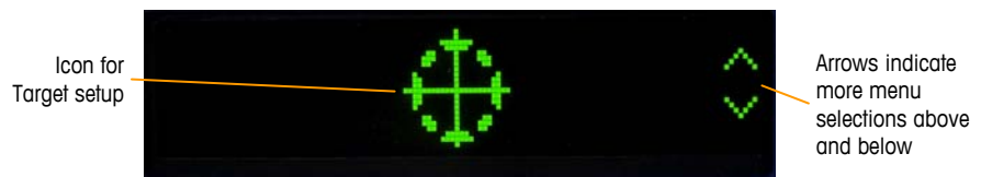
Figure 2-2: Display in Operator Entry Mode, Target Icon Displayed
