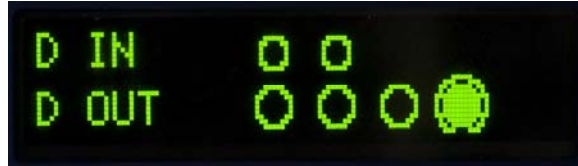
Figure 4-6: Discrete I/O Test Screen, One Output Active
