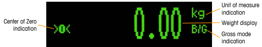
Figure 2-1: Display in Weighing Mode
