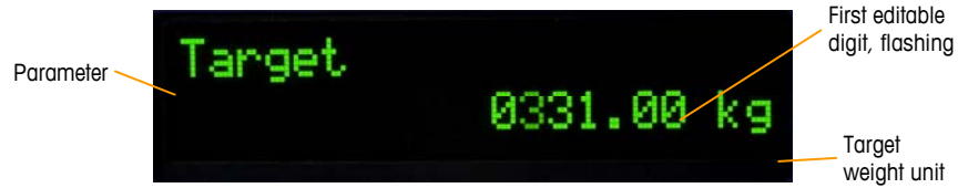
Figure 2-7: Target Entry Screen, Value in Focus
