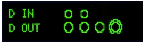
Figure 3-18: Discrete I/O Test Display, Output Active (bottom)
