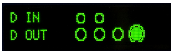
Figure 4-6: Discrete I/O Test Screen, One Output Active
